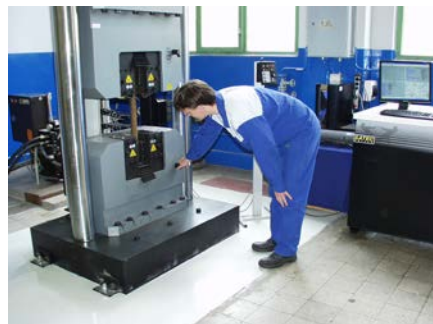
Testing of reinforcement bars
